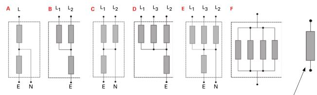
This symbol represents individual, high surge-capacity, surge protection devices, fuses capable of interrupting high (100kA AIC) prospective fault arrestor and state-of-the-art status monitoring electronics.
