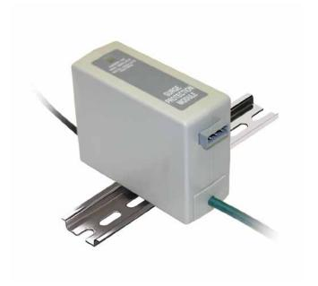
**The MA3350 is ideal for AC applications** where high surge current surge protection is needed in a small space. Typical three phase DIN rail mounting SPDs are 89mm wide, the MA3350, at 38mm wide, is a remarkable 64% thinner. Each mode in the MA3350 is rated to a full 50kA (8/20  $\mu$ s). In the three phase unit there are 4 such modes giving a total unit rating of 200kA.
