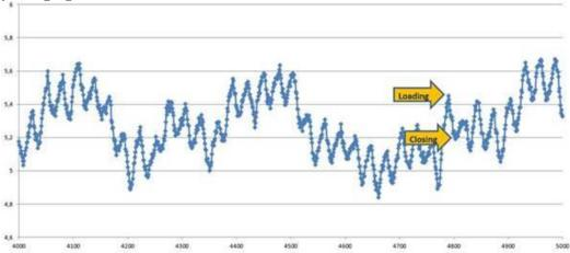
On the y-axis the oxygen value is displayed and on the x-axis the time. Out of the measurement you directly see the loading and sealing/closing of each bag. This confirms, that it is possible to measure the content of each bag.
