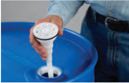
2 Place the drum insert assembly in drum.
