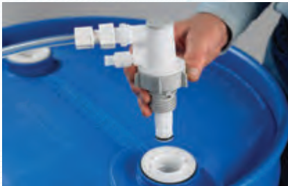
4 Insert coupler into drum insert assembly.
