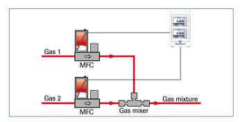
MFC's are often used to make precise and stable mixtures of two or more gases. A Bronkhorst<sup>®</sup> PS/Readout system can be applied to maintain the ratio of mixed gases by operating in master-slave mode. In the example above, the flow range of gas 1 is much smaller than the other. For this purpose Bronkhorst developed a gas mixer, to guarantee a homogeneous gas mixture.
