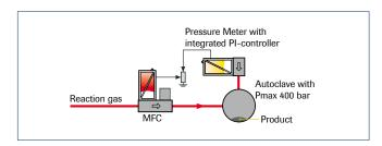
Flow control is often combined with the control of reactor pressure, using an EL-PRESS back pressure controller, or as depicted, an EL-PRESS Pressure Meter with integrated PI-controller. Typical applications: high pressure hydrogenation systems and autoclave processes using a 400 bar rated Mass Flow Controller with Vary-P control valve.
