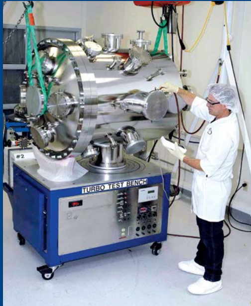
Chamber Leak Test in Class 1000 Clean Room
