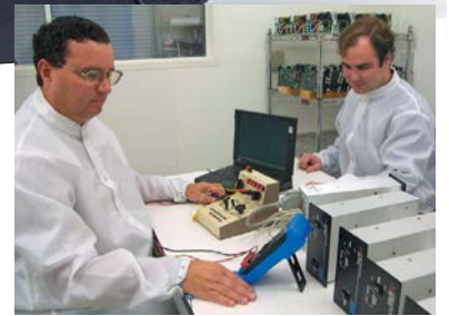
Intellisys adaptive pressure controller calibration
