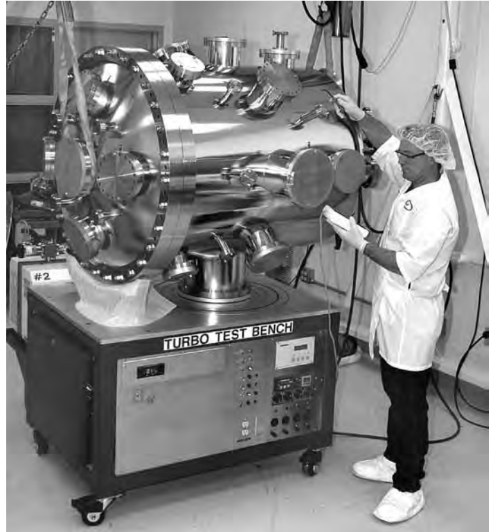
Leak testing of chamber on chamber qualification test bench
