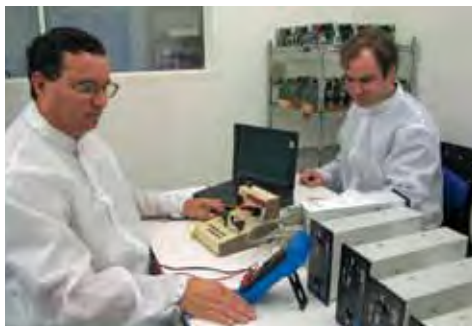
Calibration of Intellisys adaptive pressure controllers
