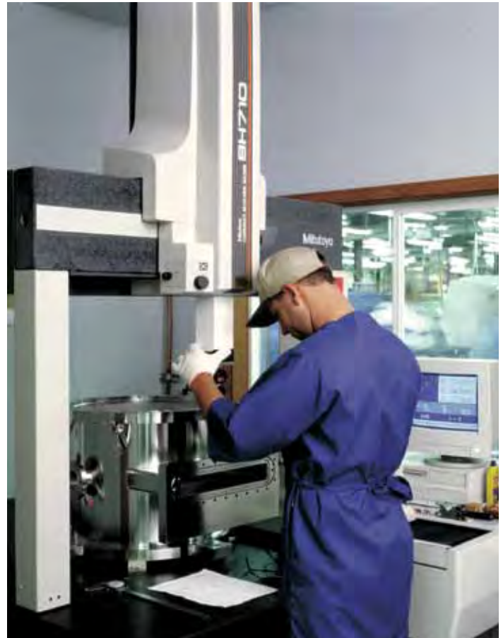
Mechanical inspection of process chamber with CMM
