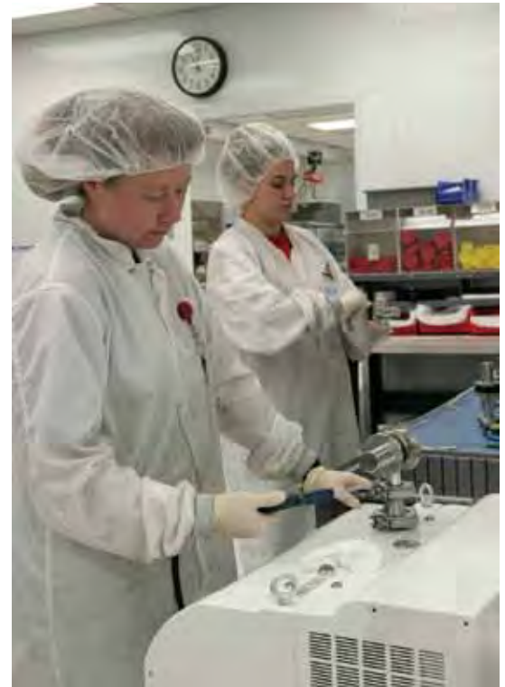
Dry leak detector for valve inspection
